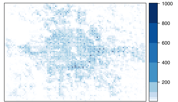
Fig. 6. Average parking demand for each cell. Colorcode represents the number of parked bikes.
